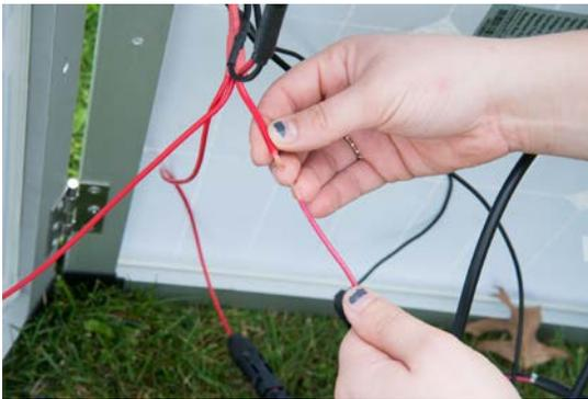
**Step 8:** Connect the negative (black) load wire from the charge controller to the negative (black) alligator clip on the negative terminal of the energizer.
