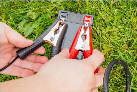
**Step 3:** Connect Panel A's negative (bottom) plug to the charge controller's negative (black) plug.
