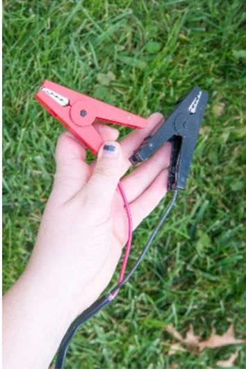
\*Remove the alligator clips from the energizer, and mark the positive and negative wires prior to removal. Strip the insulation from the wire ends. Splice the alligator clip ends to the corresponding charge controller load wires.
