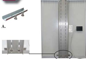
Use two bolts to install the channel clamp to bottom of solar panel. The channel clamp fits between the frame of the solar panel and the panel bracket with the large flat side facing the solar panel. Bolts fasten via the slots on the panel bracket.
