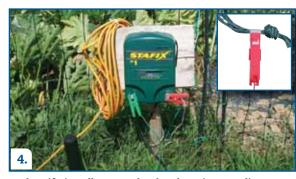
To electrify, install a ground rod and use jumper clips to connect the net to an energizer (low impedance, minimum .25 joule per net) or to an existing electric fence.
